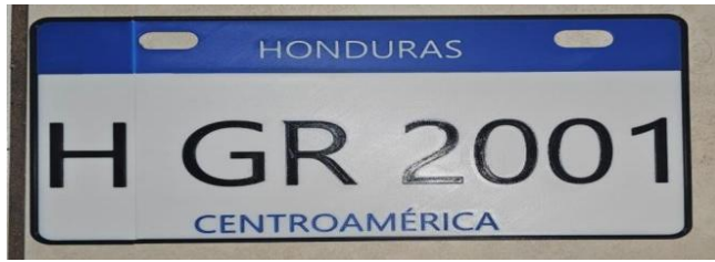
Fig. 5 Final result of printing vehicle license plates in 3D printing.
