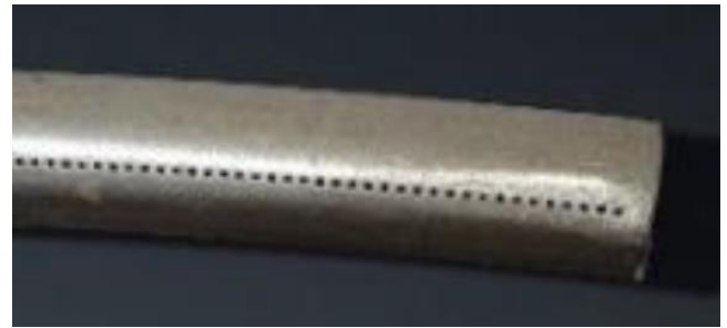
Figure 3. Part of a closed end perforate tube used in an impingement cooling system.
