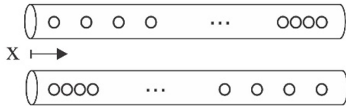
Figure 16. Two scenarios for non-uniform distribution of equal-size holes ( g_d = 15 ).
