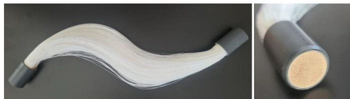
Figure 1: Bundle of hollow-fiber membranes with detail of potting.
