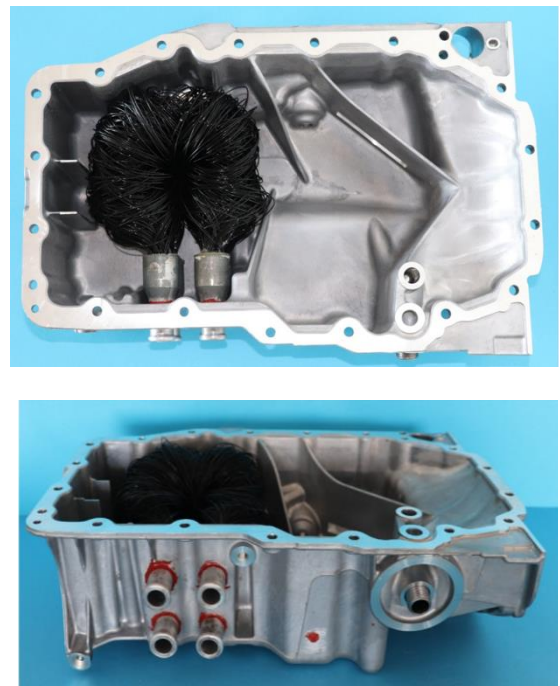
Fig. 4: Polymeric hollow fibre heat exchanger in the engine oil sump.
