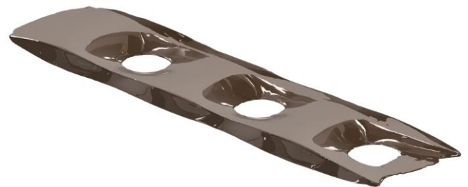
Figure 5: Interpolation of the internal volume of a slice cut from the SSPPHE plates and from the mesh obtained by tomography
