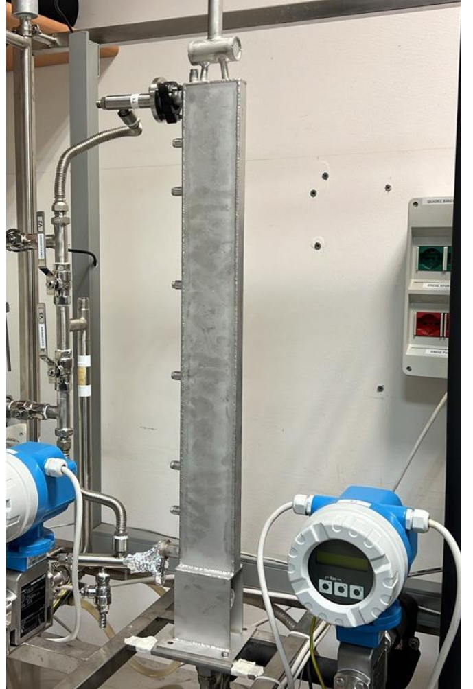
Figure 1: Detail of the SSPPHE prototype mounted on the experimental set-up, prior to thermal insulation.
