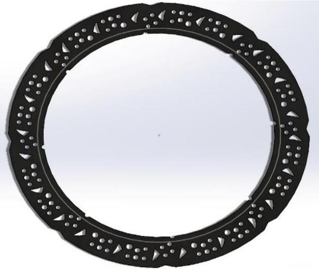
Figure 3. Extruded brake rotor used for the thermal analysis.
