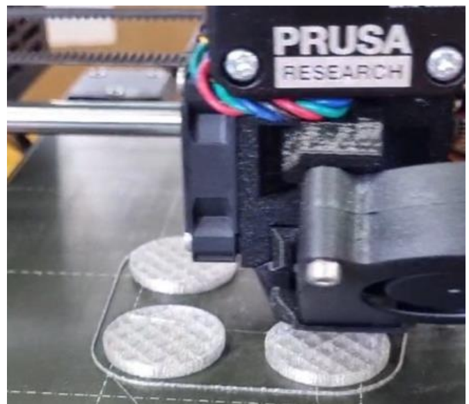
Figure 3: Pilot Printing of Test Specimens.
