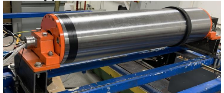
Figure 4. Test rig constructed for the estimation of viscous dissipation inside the electrical motor.
